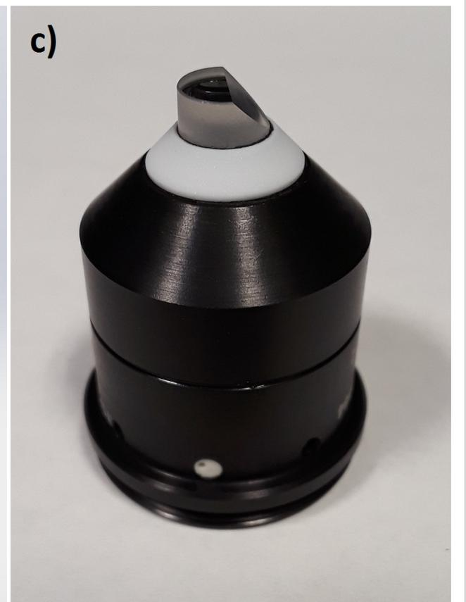
**Figure A1: Bespoke glass-tipped objective AMS-AGY v1.0.** A drawing a) shows the critical opto-mechanically coupled design considerations for the bespoke objective: to collect a tilted air space image just
