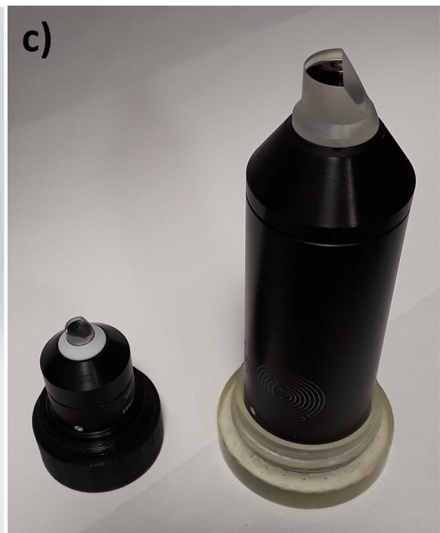
**Figure A2: Bespoke glass-tipped objective AMS-AGY v2.0.** A drawing **a)** shows the critical opto-mechanically coupled design considerations for the bespoke objective: to collect a tilted air space image just ~16µm from a flat surface, with a range of tilt angles from 0-55 degrees. A CAD rendering **b)** of the v1 and v2 designs side by side and a photo **c)** of the v1 and v2 final working lenses.
